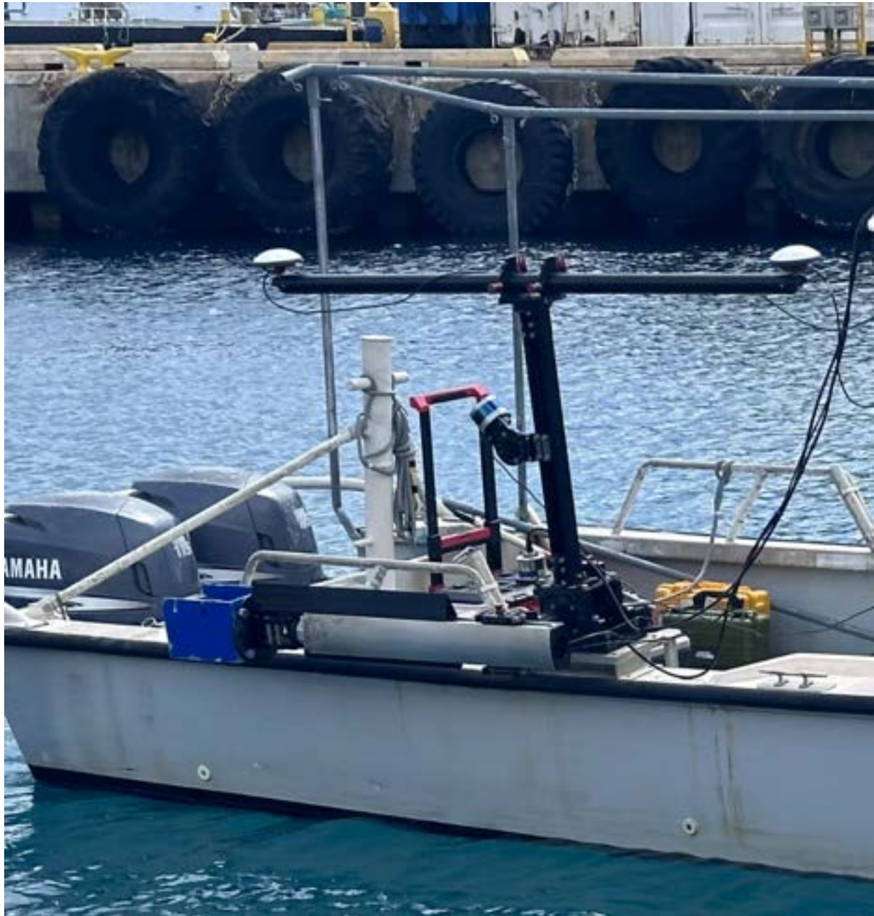
Figure 2-2. Vertical MBES pole mount, shown as installed, with RTK GNSS position antenna on top, and LiDAR puck.
